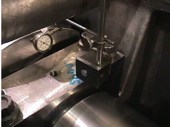
Dial Indicator Magnetic Stand Placement on Top of Main Bearing Cap
