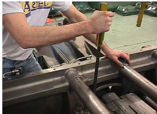
Use a Pry Bar against Compressor Frame, Thrusting Crankshaft Back & Forth
